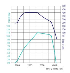
**4P10 – 110 kW (150 PS)** 400 Nm@1600 rpm 110 kW@2626 rpm
